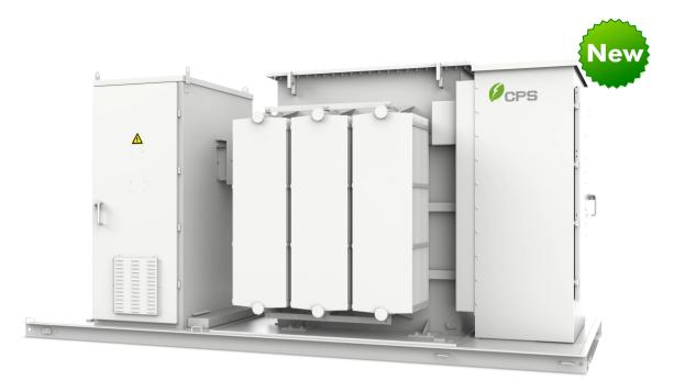
The CPS three-phase 4.2 MVA Medium-Voltage Transformer Skid Solution is the last step in the conversion chain that brings electrical energy to the power grid. The transformers are designed for superior reliability, efficiency, and environmental performance. A modular architecture paired with design options ensures cost efficiency and easy, minimal maintenance. The Skid Solution includes the Low-Voltage Cabinet, Auxiliary Transformer, communications and controls.
